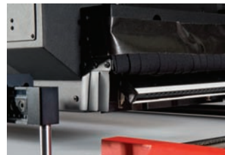
Shuttle safety sensors prevent printheads from touching the substrate. The ionizer bar avoids electro static loads. Both are located on the shuttle.
